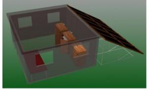
The sketch below shows approximate size of the small building and interior space required for three Quad series collectors and their respective cabinets in the building.
