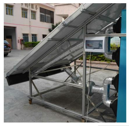
То maximize airflow efficiency. Quad the series draws air downwards through the solar air collectors to allow the hot air outlet ducts to be directed into cabinet. This can also be done either from a rooftop installation or from the ground outside a small building. The photo at left shows the manifolds. ducts and fans coming off the Quad collectors, and the control panel.
