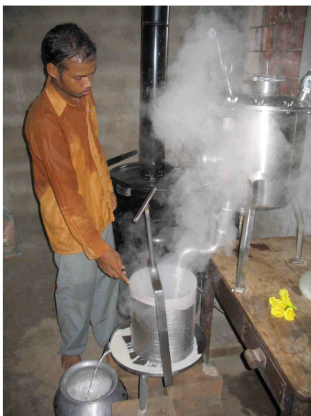
Soymilk production in Orissa, India, showing cooker (on table) and press below with boiler at rear.
